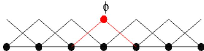
A finite element basis function in 2D
